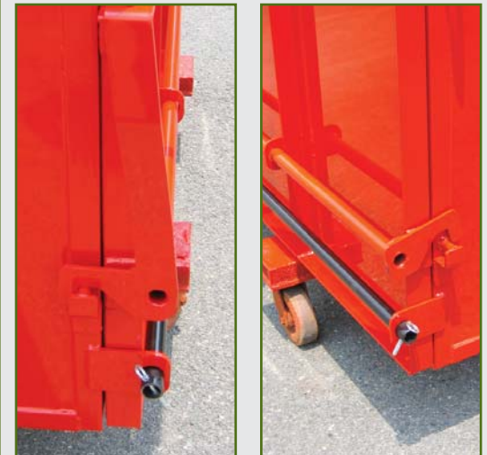
Easy to open and close latch mechanism makes closing the door simple and virtually effortless. No more binding or pinched fingers.
