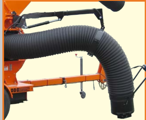
Maneuvering the hose boom is almost effortless because the boom is raised and lowered hydraulically using push button style switches and the boom swivels side to on two flange bearings.
