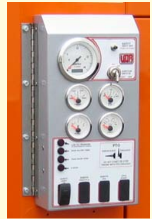
Hinged instrument panel allows easy access to the instrument wiring. All engine monitoring gauges are backlit for increased visibility.
