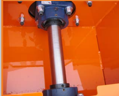
The drive bearings assembly consists of two heavy-duty four-bolt flange bearings with double row, precision spherical roller bearings. The entire assembly can be removed in one piece by removing eight bolts. This is a major labor and cost savings feature.
