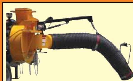
Hydraulic hose boom is standard and maneuvering the the hose is almost effortless because the hose is raised and lowered hydraulically and swivels side to side on flange bearings.
