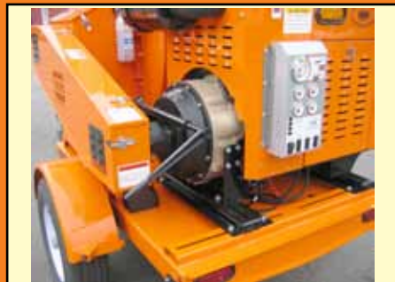
The PTO/Clutch is a heavy duty 13" automotive style assembly with safety engagement system.
